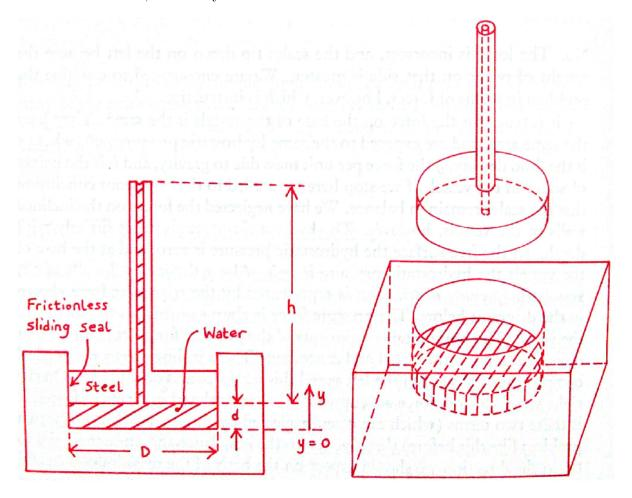
(a) Calculate the equilibrium height of the water in the tube (measured from the bottom surface of the piston).
