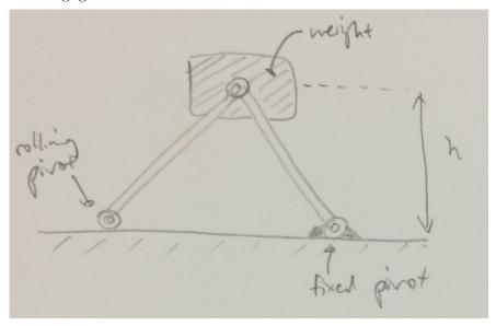
The rods are pivoted (like an elbow joint) at both ends. One rod has its bottom end pivoted to a fixed pivot on the floor, while the other rod has its bottom end pivoted to a rolling pivot that can move along a straight horizontal track.
