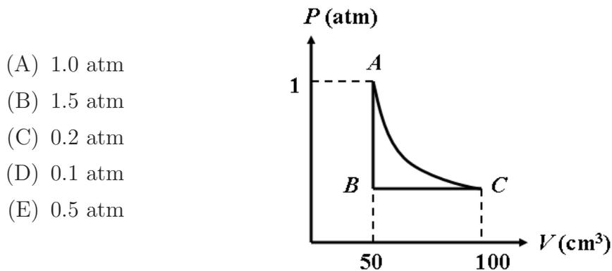
20. A thermodynamic system undergoes a cyclic process as shown in the figure below. The heat energy absorbed by the system over one complete cycle is:
