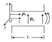
A stream of charged particles, each with charge q, is ejected at y=z=0 at various positions along the x-axis. The particles each have an initial momentum of  $p_0=p_0\hat{z}$ , where  $p_0\gg qLB_0$ . Show that the charged particles are focussed to a point, and find the z-coordinate of this point.
