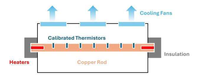
Internal Experimental Setup
