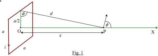
At O, the centre of coil, the magnetic field for a single turn is
